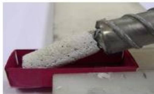
Drill Tool with sample acquisition mechanism
